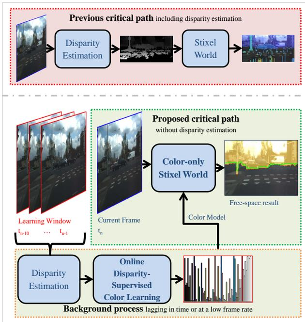
Fig. 2. A comparison between the existing and our proposed framework. Previous systems [1][7] require disparity estimation in their critical path, in contrast to our proposed system. Note that our disparity-supervised color modeling in the lower part of the scheme can be lagging or run at a lower frame rate than the critical path, by varying the range of the learning window.
