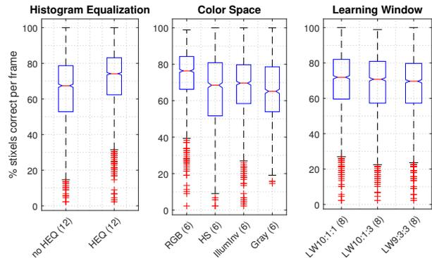
Fig. 3. Box plots comparing the different settings over all runs. For each frame in each run, the percentage of stixels with a correct free-space estimate is calculated, which is visualized as a box plot per setting. Hence, each box contains 188 data points per run. The number of runs per box is denoted in brackets in each label.
